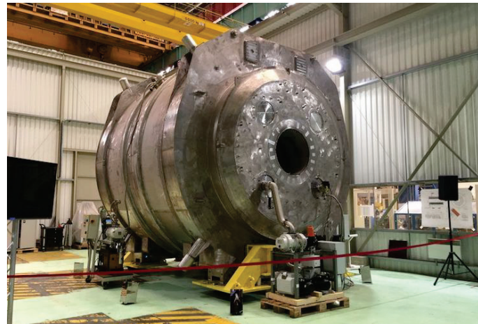
Iseult magnet, 11.75 T, ~150 tons 5m outer diameter
